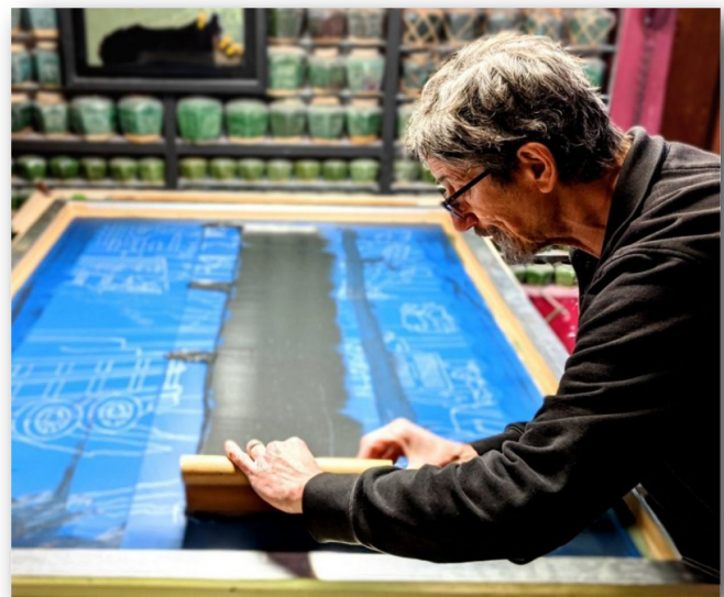
Richard is employing the cuerda seca tile making technique. The line artwork is photo exposed onto silkscreens and a waxy medium is used to transfer the lines onto ceramic tiles.
