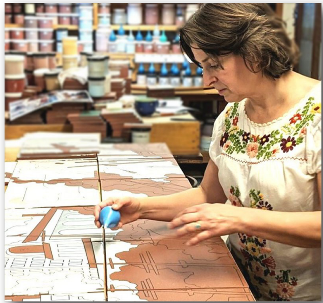
At left: the screen has been successful in transferring the line drawing to the tile surface. Above: Mary bulbs the various colored glazes onto the tiles. Below: A portion of one of the murals glazed and ready for firing.
