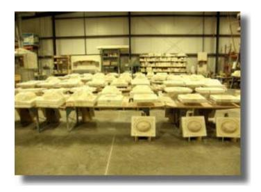
Here are many of the molds used to produce Marzi sinks.
